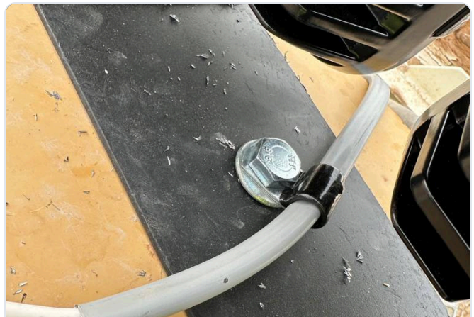
Rubberized clamp holding a run tight to the frame.
